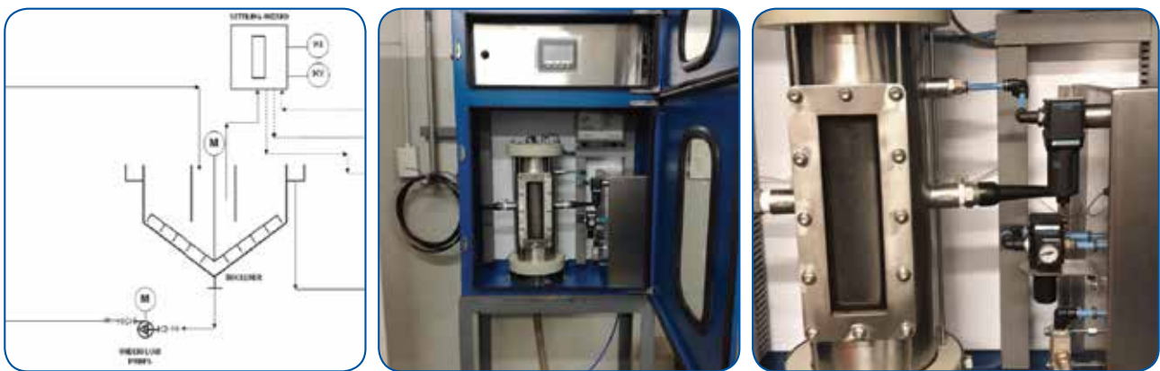
Figure 2: P&ID of typical Settling Wizard installation
